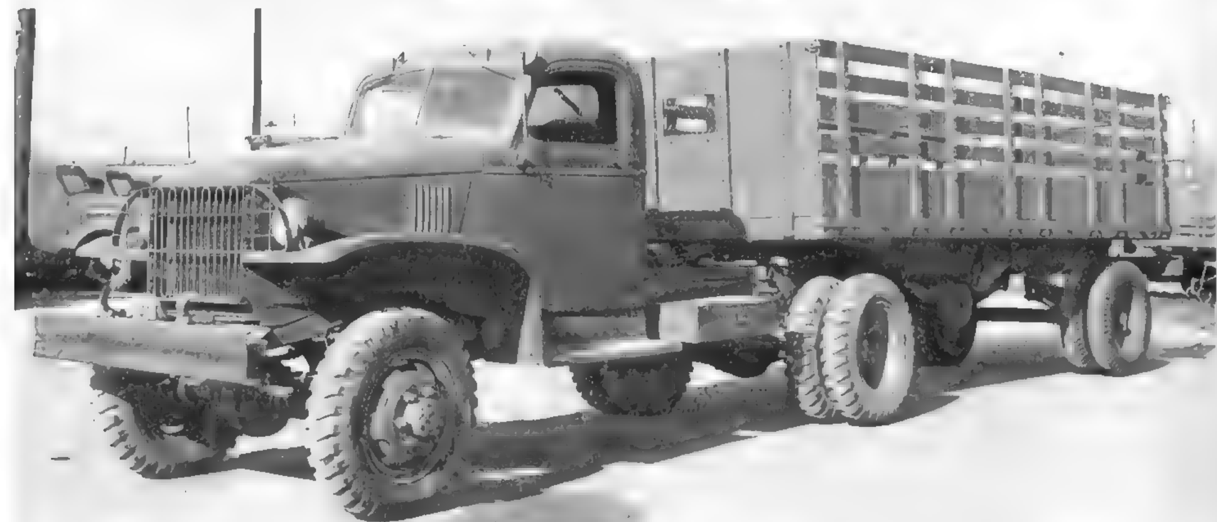
Coupled here to a 6-ton trailer, the G7113 Chevrolet was used as light general-purpose truck tractor, a role many of them served in on the surplus market as well. (National Archives and Records Administration photo)
